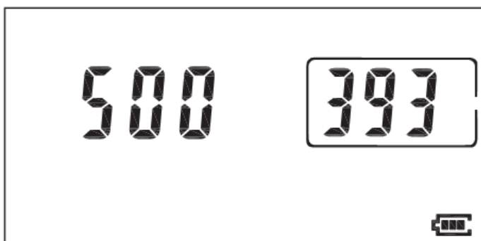
Example 2: Trailer ID (500393) and a flashing trailer.
